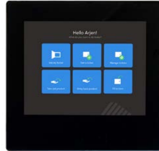
The screen can be used to open the compartments and to provide information on the content
